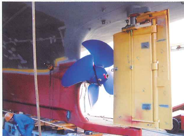
プロペラ取付け / Fitting of propeller in rudder
