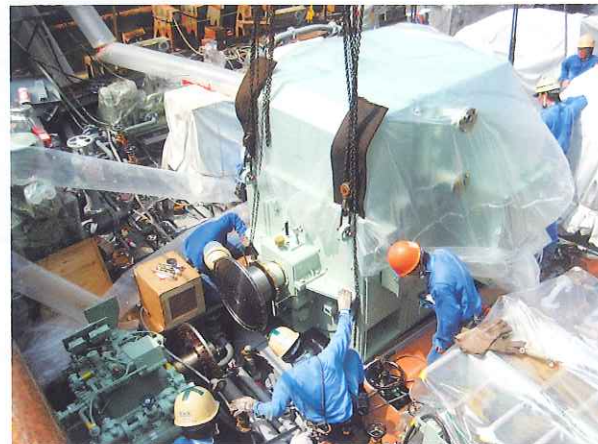
減速機及び推進電動機搭載 Installation of reduction gear and propulsion motor
